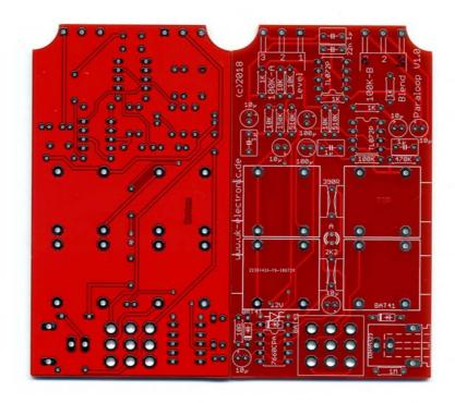
The printed resistor 150k must be 510k!!
